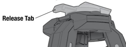
1. Position the open end of the Dove Tail Mount **9** at the release-tab side of the tripod (see the picture above).
