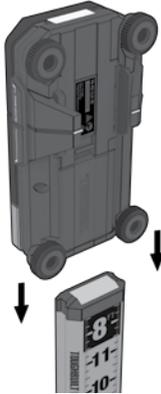
2. Squeeze the two brake release pads **21** and lower the receiver until the top of the grade rod clears the upper rollers.
